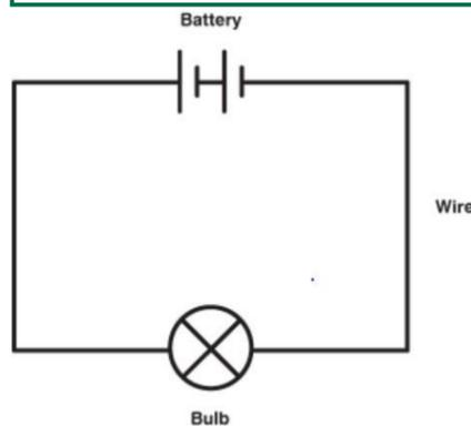
In order for electricity to flow, a circuit needs three things:
